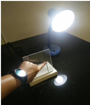
Demonstrate of Transparent Hybrid Touch Switch
